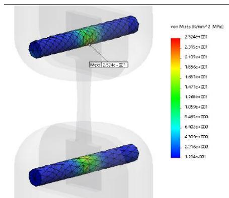
**Figure.4: Stress Concentration result of Pin For Al 6061**
