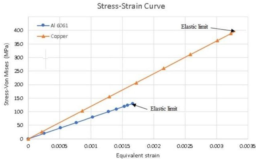
Fig. 9 Stress - strain curve for aluminium 6061 and copper
