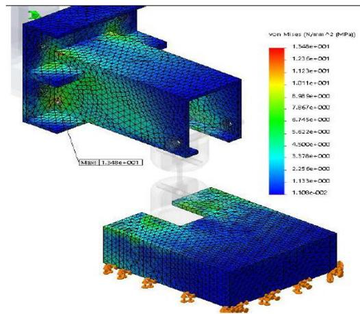
**Fig.6 Stress distribution on the grip holder for AL 6061**
