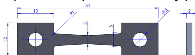
**Fig.7 Dimensions of specimen**
