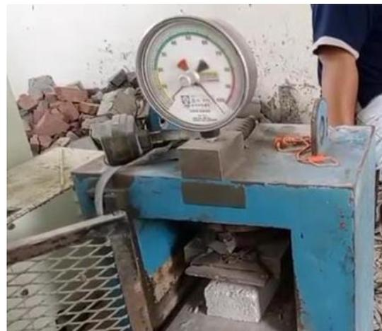
Figure 3. Compressive test of paving block
