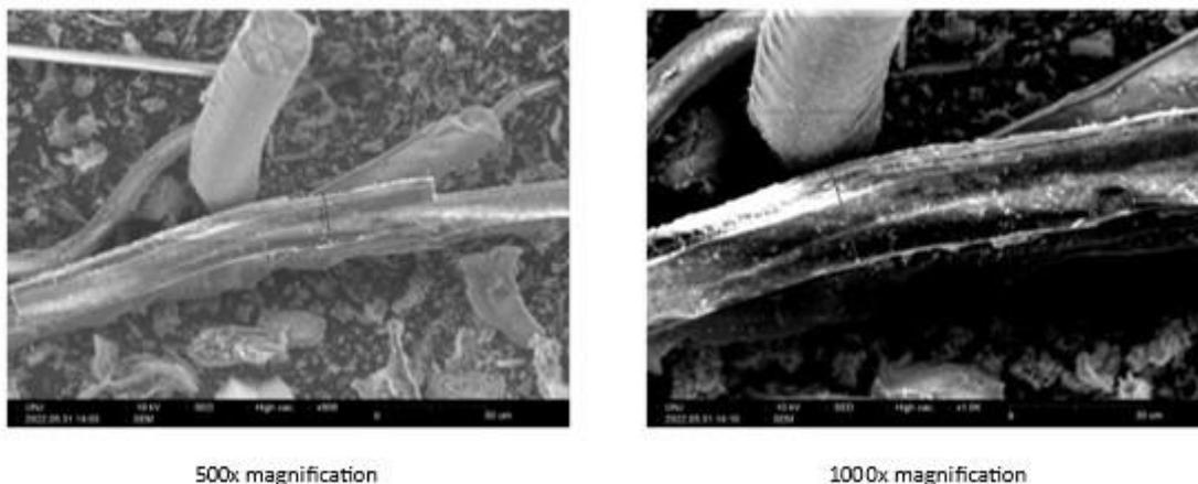
Figure 4. SCBA with final calcination temperature of 600°C
