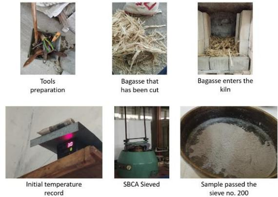
Figure 2. Sample preparation process
