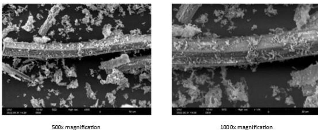
Figure 5. SCBA with final calcination temperature of 700°C
