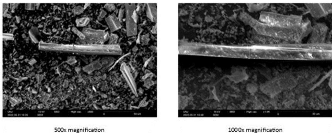
Figure 3. SCBA with final calcination temperature of 500°C
