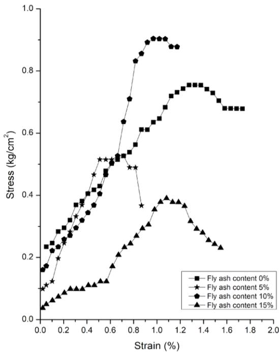
Figure 3. Stress-strain relationship obtained from UCT
