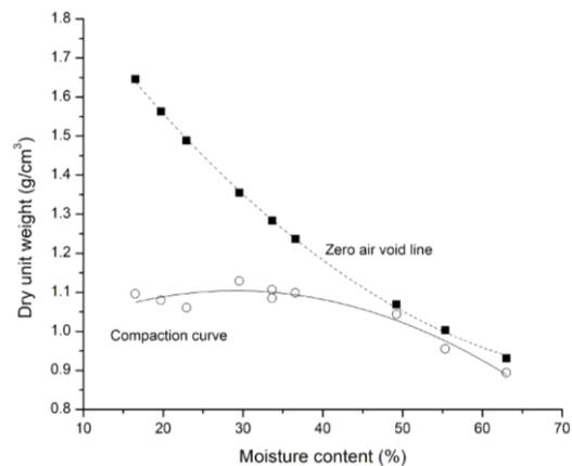
Figure 2. Compaction curve and zero air void line
