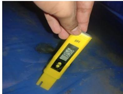
Figure 3. Seawater pH measuring
