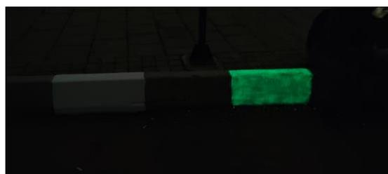
Figure 3. Comparison of Phosphorescent Paint and Regular Paint at Night
