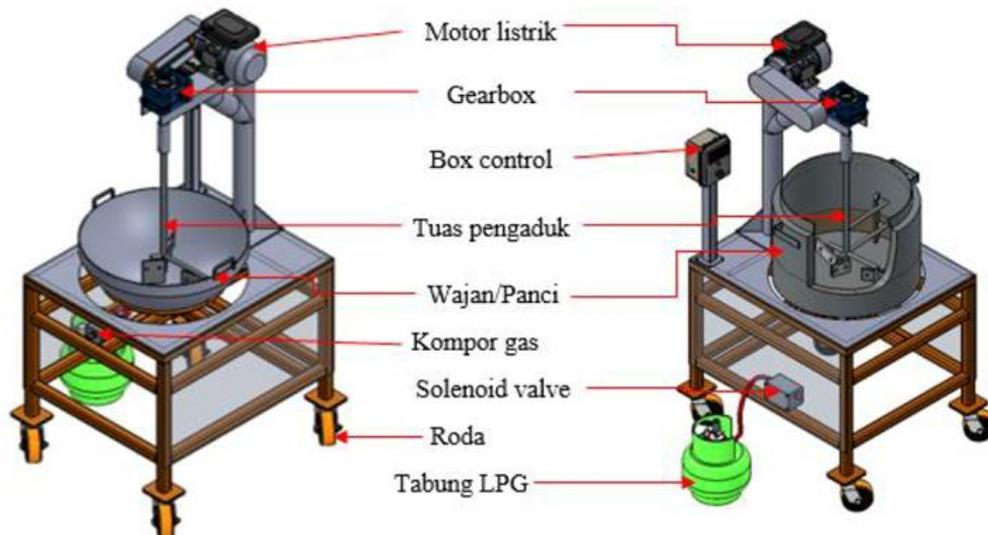
Figure 1. The design of the shrimp paste mixer machine
