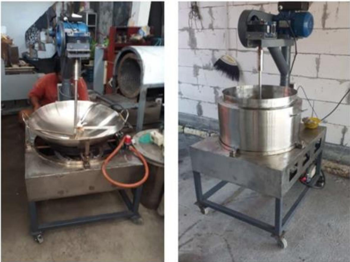
Figure 2. The temperature-controlled shrimp paste mixer machine
