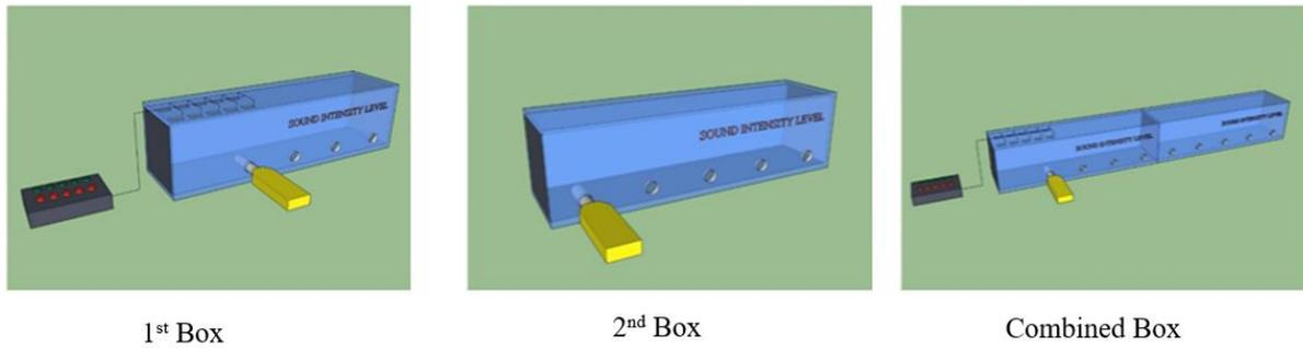
**FIGURE 2.** Design of the Sound Variable Intensity Level Kit
