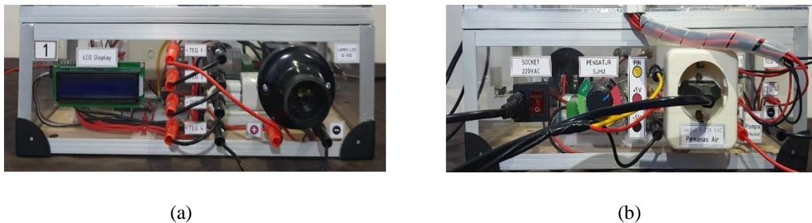
**FIGURE 5.** The components of electricity bodies in the IoT-based thermodynamic law experiment media (a) front view and (b) rearview.
