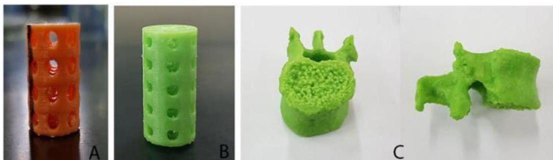
FIGURE 7. 3D prints. (A) NaCl template with 4 holes. (B) NaCl template with 5 holes. (C) Vertebrae bone.
