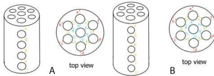
**FIGURE 1.** NaCl template for material research apparatus. (A) Design 4 holes. (B) Design 5 holes.
