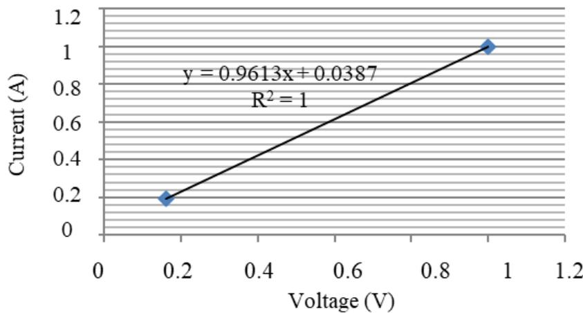
**FIGURE 4.** The Relationship of Voltage (V) and Current (I) in a Parallel Circuit
