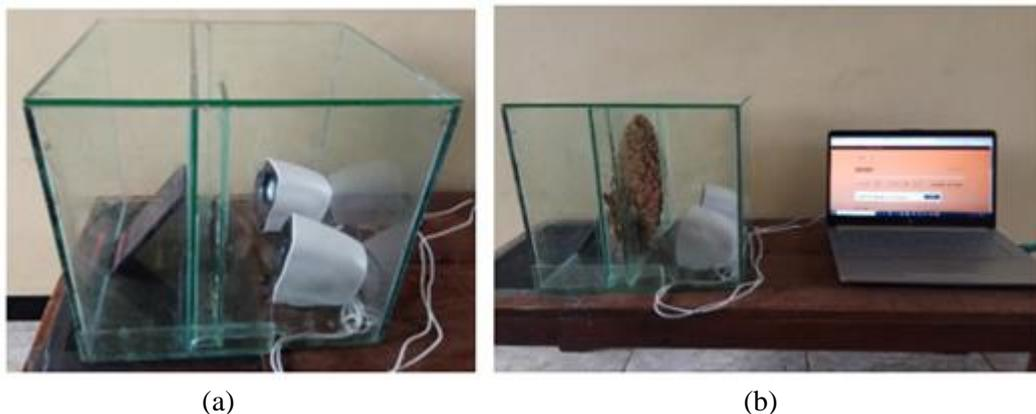
**FIGURE 5.** (a) Setting for data collection using a glass slide, (b) Setting data collection using a glass slide plus a water hyacinth placemat sample
