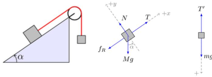
**FIGURE 2.** A block on the ramp and FBD of block
