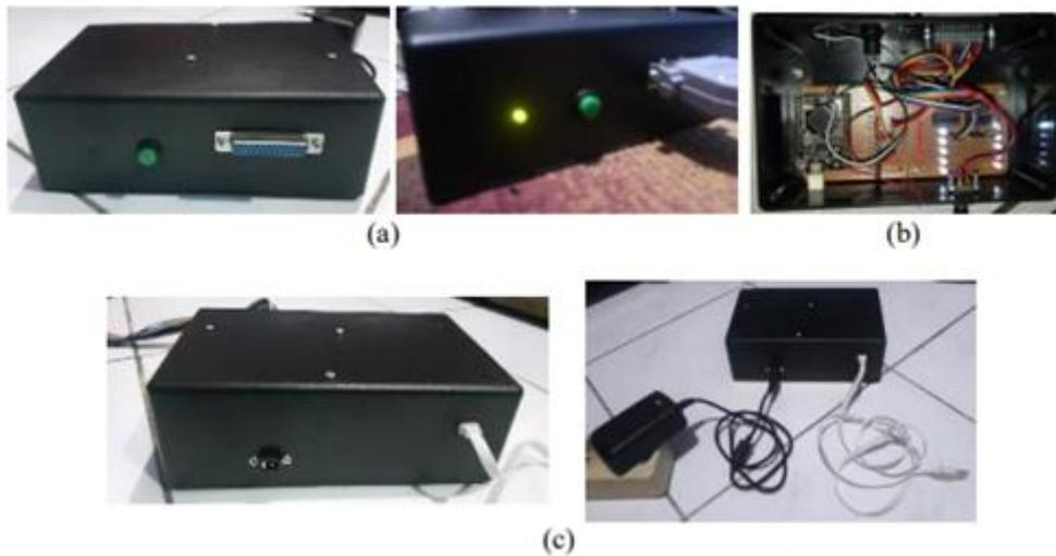
**FIGURE 5.** (a) Front view, (b) Contents of the electronics box, (c) Back view
