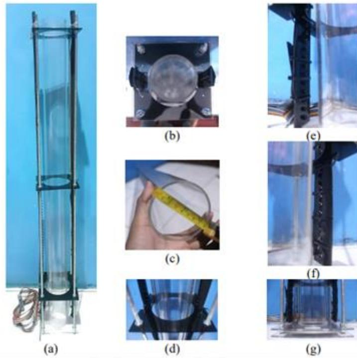
**FIGURE 4.** (a) Overall view, (b) Top view, (c) Trajectory tube, (d) Holder, (e) Photodiode sensor, (f) Infrared sensor, (g) Bottom view of the track frame
