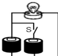
In the circuit below, the two batteries are identical and ideal (no internal resistance). The electric current in the circuit when switch S is disconnected is I
