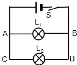
In the circuit above, the battery is ideal (no internal resistance) and the lamp is identical. When switch S is connected, the electric current through the lamps L<sub>1</sub> and L<sub>2</sub> is the same
