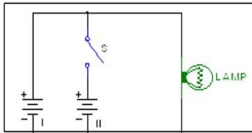
The following question concerns addition voltage source (battery) in the circuit electricity. L lamp arranged with source voltage I, voltage source II arranged in parallel as shown in the figure below. Second source is the same and ideal, meaning that the voltage remains regardless of the electric current
