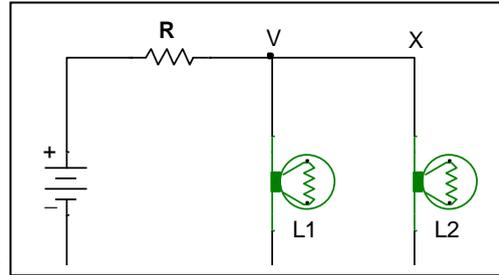
16. If lamp L<sub>2</sub> is removed from its place, the electric current through lamp L<sub>1</sub> will be:
