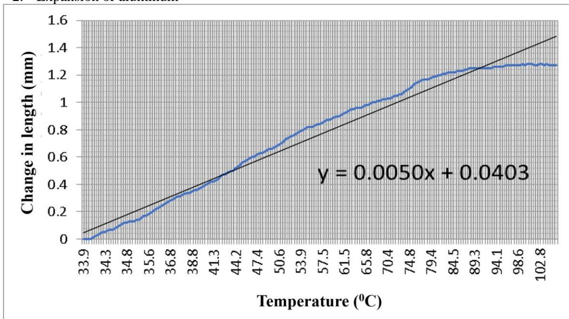
**FIGURE 6.** Graph of thermal expansion results on aluminum bars
