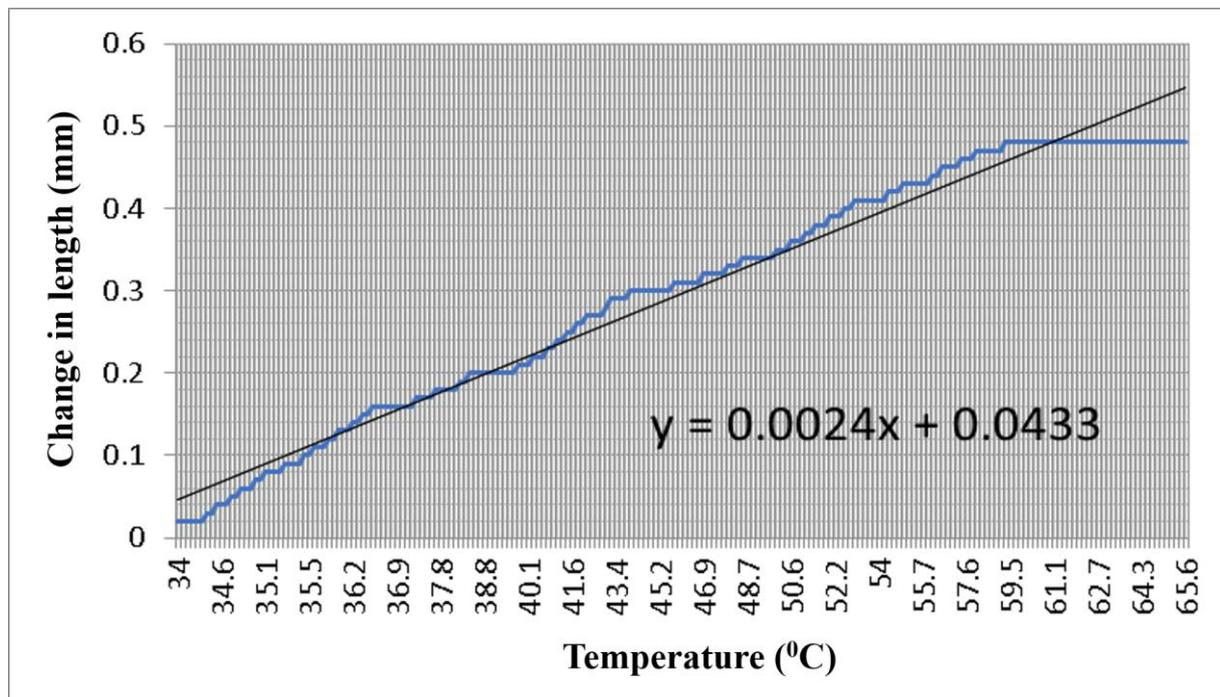
**FIGURE 5.** Graph of thermal expansion results on iron bars
