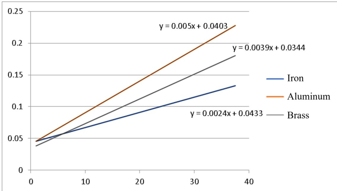
**FIGURE 8.** Graph  $\Delta L$  relationships with  $\Delta T$  of three different metal bars
