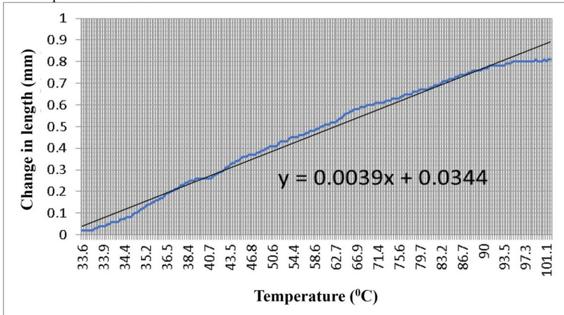
FIGURE 7. Graph of thermal expansion results on brass bars
