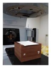
GAMBAR 1. Rangkaian Kalibrasi Film Gafchromic EBT3.
