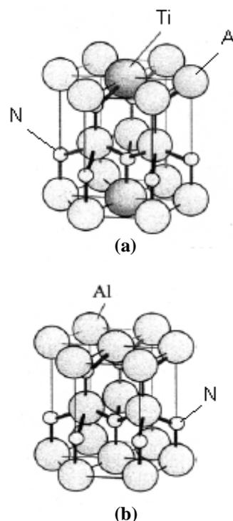
**Figure 2** Model schematic of (a) hexagonal-TiAlN; (b) hexagonal-AlN [17].
