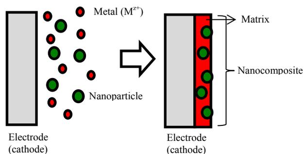
**Figure 3.** Electrodeposition of nanocomposite
