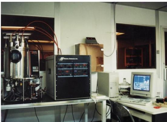
**Gambar 6.** Peralatan Sistem Sputtering ARC-12M
