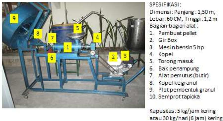
Gambar 1. Mesin pellet ikan alternative bergranulator
