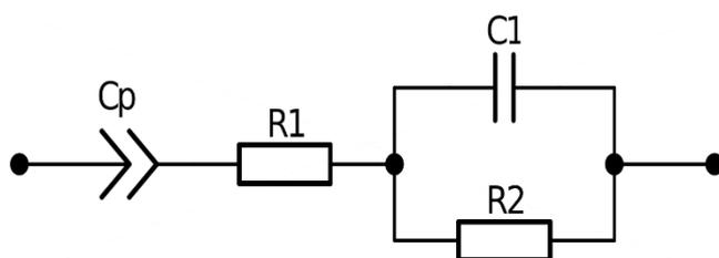
FIGURE 1. The equivalent circuit of solution.
