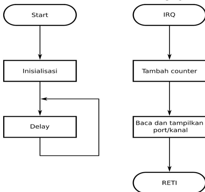
**FIGURE 3.** Flowchart of software of fry counter system.
