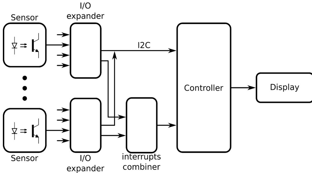
**FIGURE 2.** Block diagram of the electronics system.
