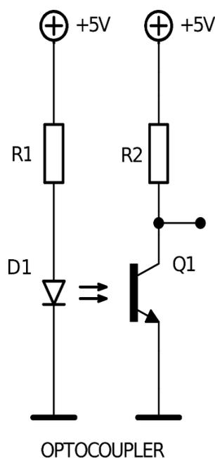
**FIGURE 1.** Opto-coupler sensor schematic.
