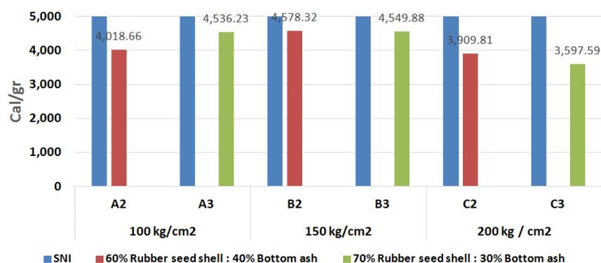
FIGURE 5. The calorific value of rubber seed shell - coal bottom ash briquettes.
