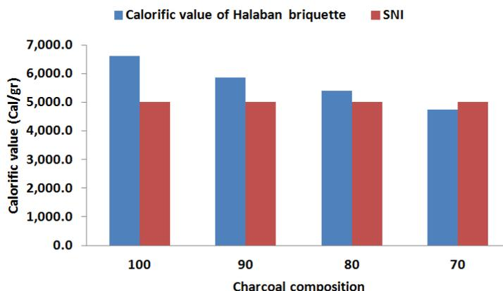
**FIGURE 6.** The calorific value of Halaban wood charcoal and coal bottom ash briquettes.
