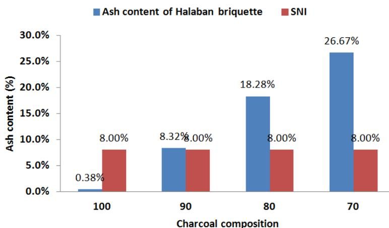
**FIGURE 4.** The ash content of Halaban wood charcoal and coal bottom ash briquettes.
