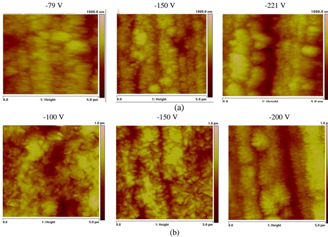
FIGURE 1. The surface morphology of sputtered TiAlN coatings at snitrogen flow rate of (a) 65 sccm (b) 30 sccm.
