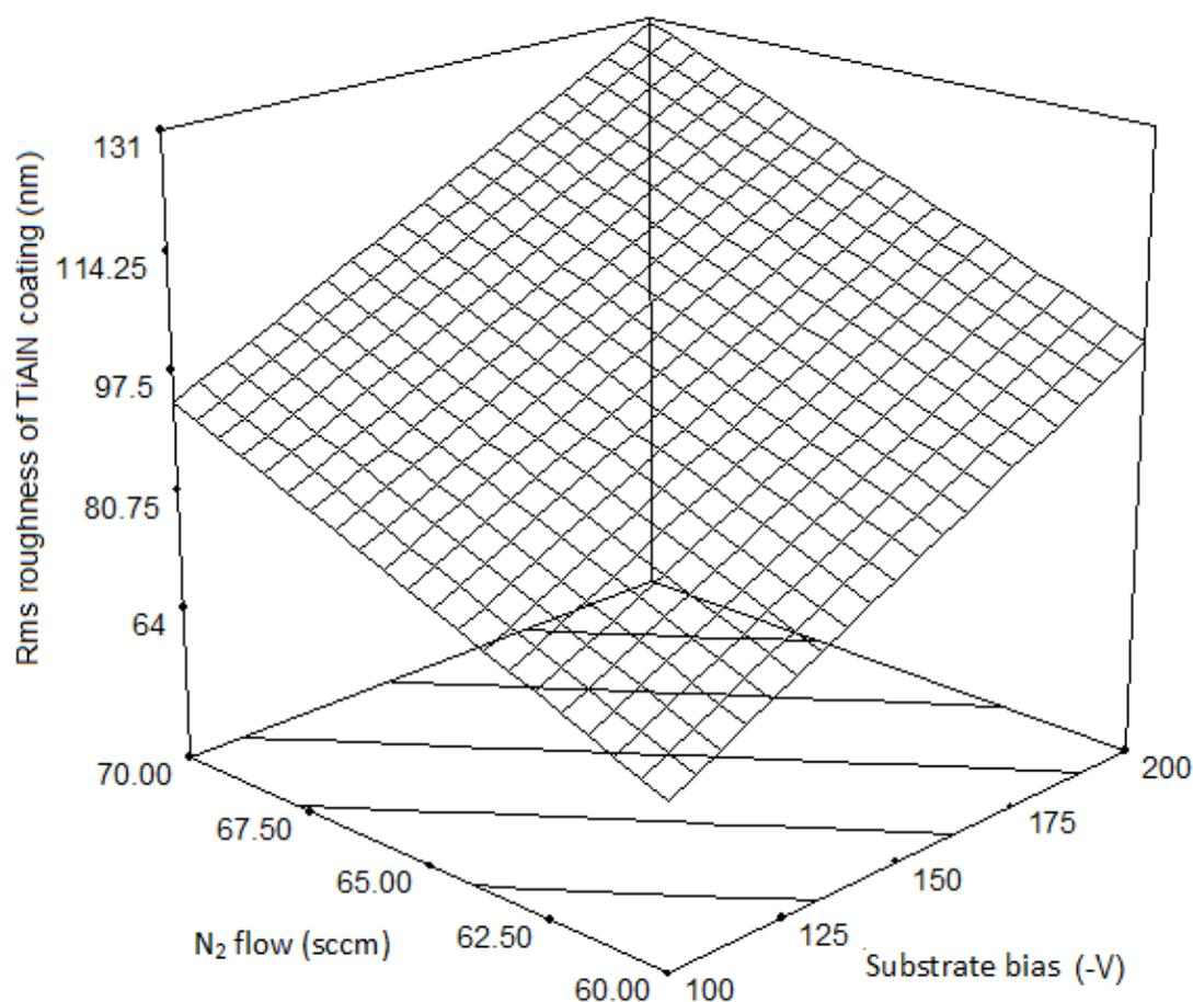
**FIGURE 3.** Three dimension graph of RMS roughness of sputtered TiAlN coatings as a function of negative substrate bias and nitrogen flow rate fall.
