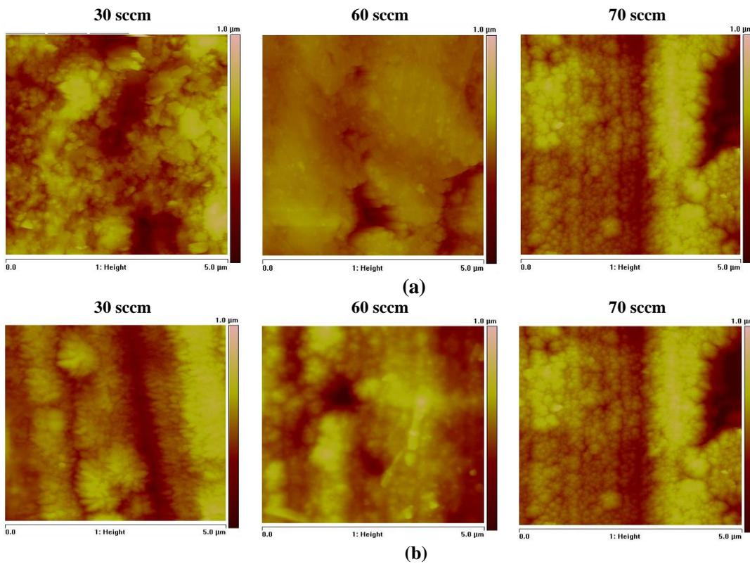
FIGURE 2. The surface morphology of sputtered TiAlN coatings at substrate bias of (a) -100 Volt (b) -200 Volt.
