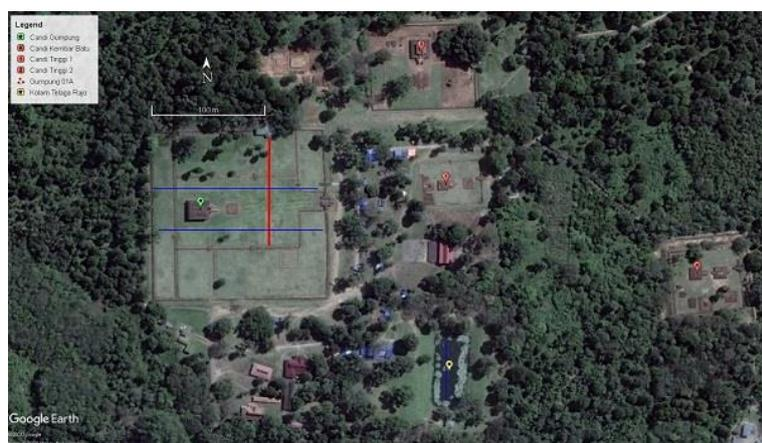
**FIGURE 6.** Location of GPR data acquisition; Gumpung Temple show with green balloon symbol. Two parallel blue lines West-East direction on Gumpung are Line 01-A and Line 02. Telago Rajo Pool show with yellow balloon symbol. Blue line at Telago Rajo Pool is Line 04.
