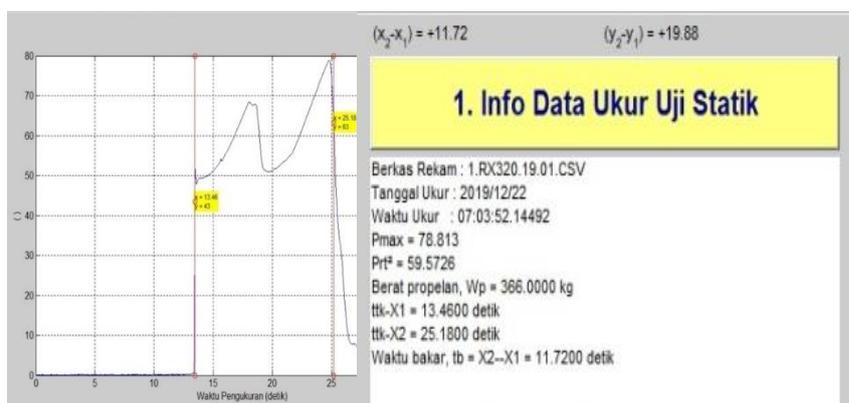
FIGURE 5. Numerical Data Acquisition Result of Combustion Chamber Pressure from Static Test of RX320.
