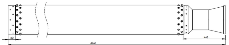
**FIGURE 3.** Technical Drawing of Rocket Motor of RX320
