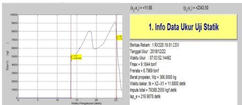
FIGURE 4. Numerical Data Acquisition Result of Thrust from Static Test of RX320.
