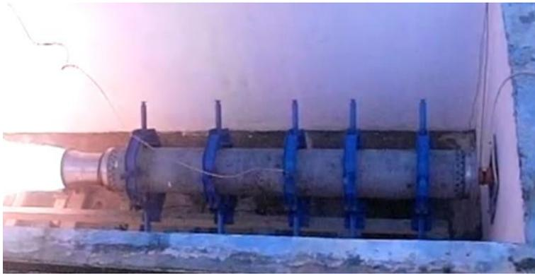
**FIGURE 2.** Static Test of Rocket Motor (Static Fire Test)
