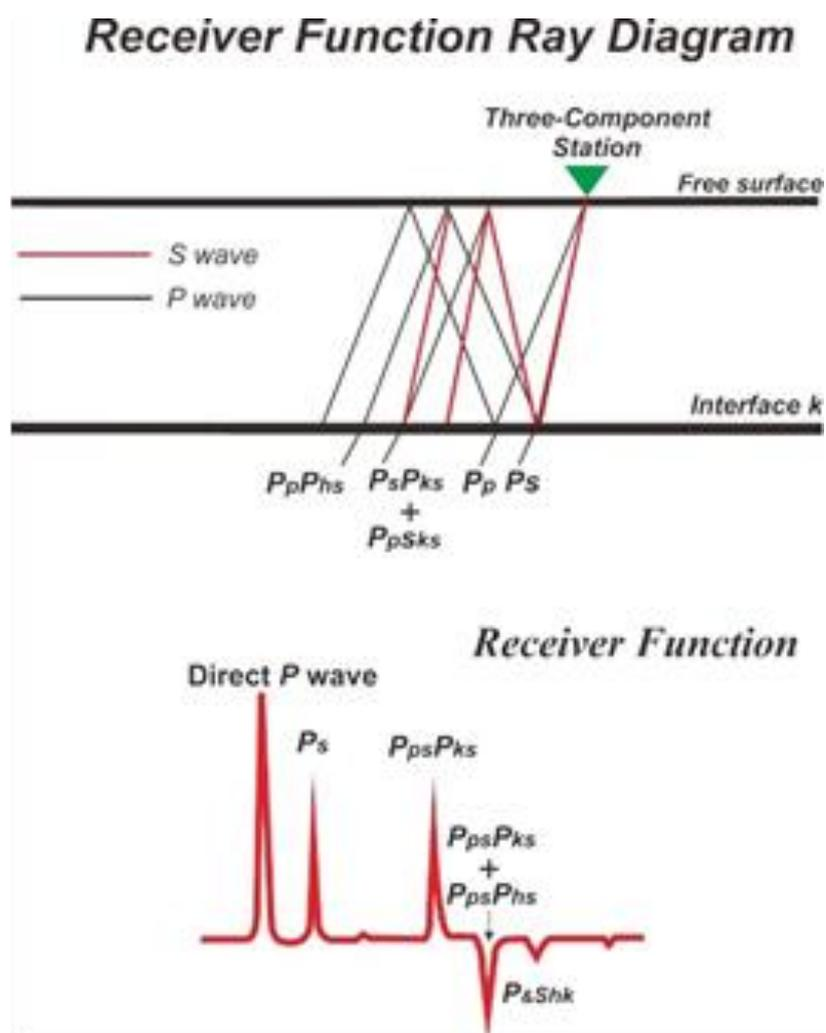
**FIGURE 3.** The simple wave propagation diagram to identifying conversion phase of P wave [9].
