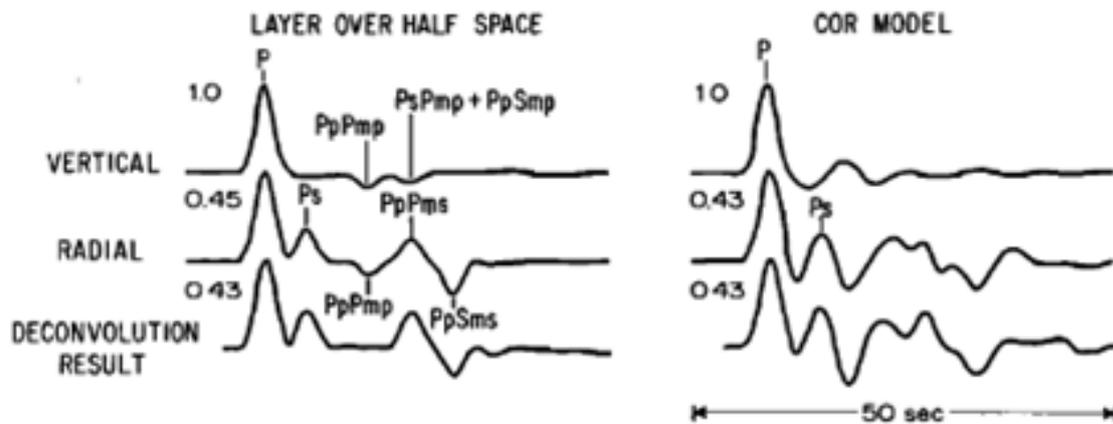
FIGURE 2. Deconvolution tecnic using two planes earth's layer (Langston, 1979)
