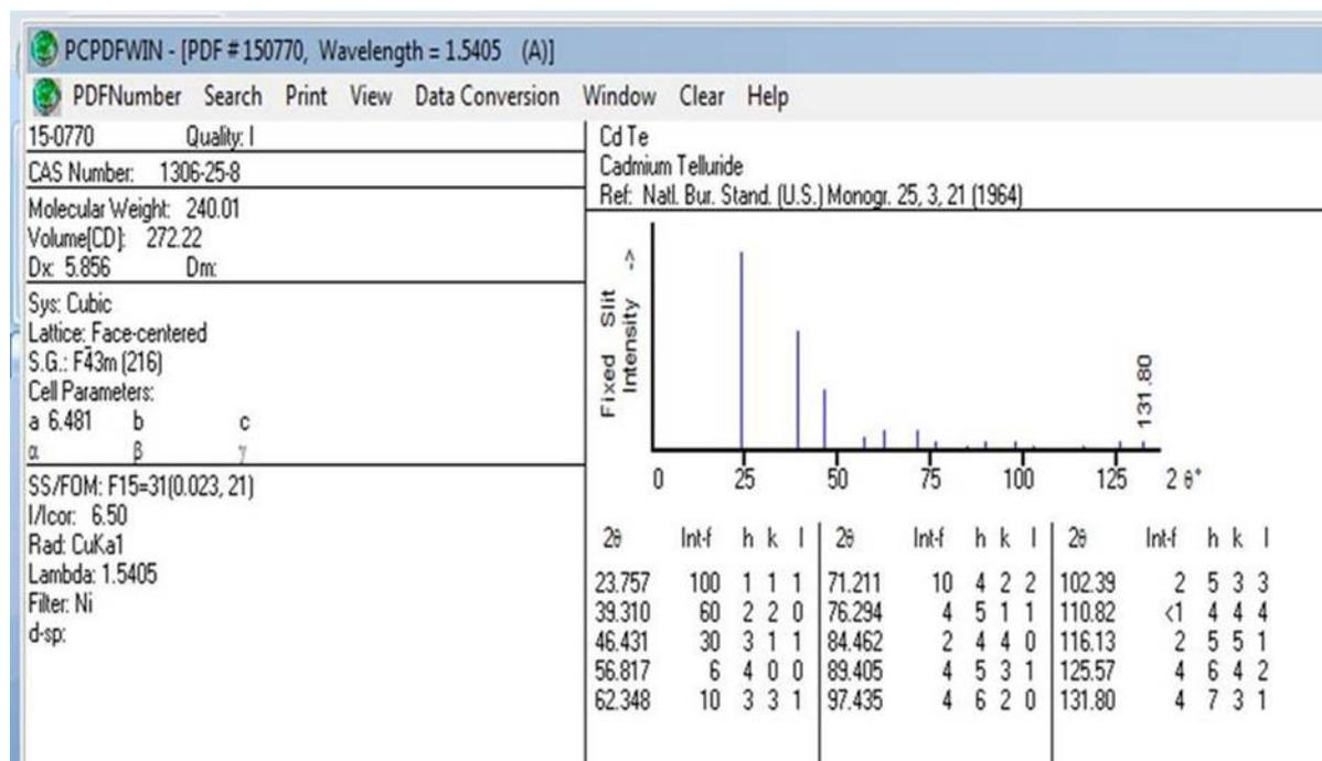
FIGURE 1. ICDD Cadmium Telluride (CdTe)
