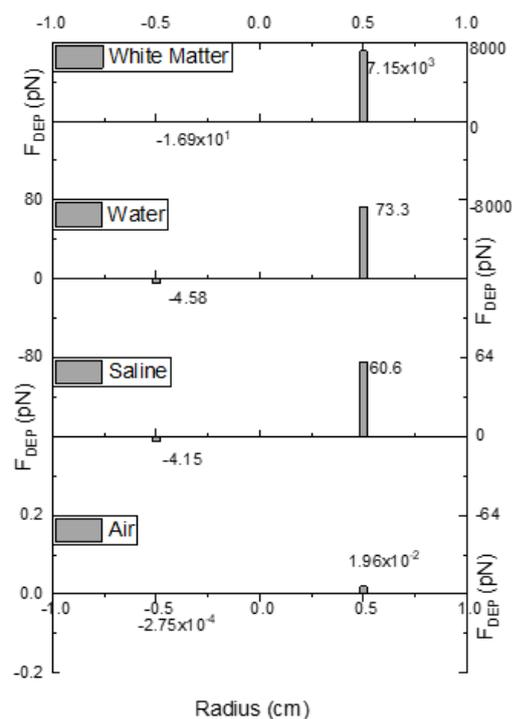
**FIGURE 6.** Dielectrophoretic force at lesion with the radius of 1 cm in various mediums placed between electrodes with an applied voltage difference of 20 Vpp
