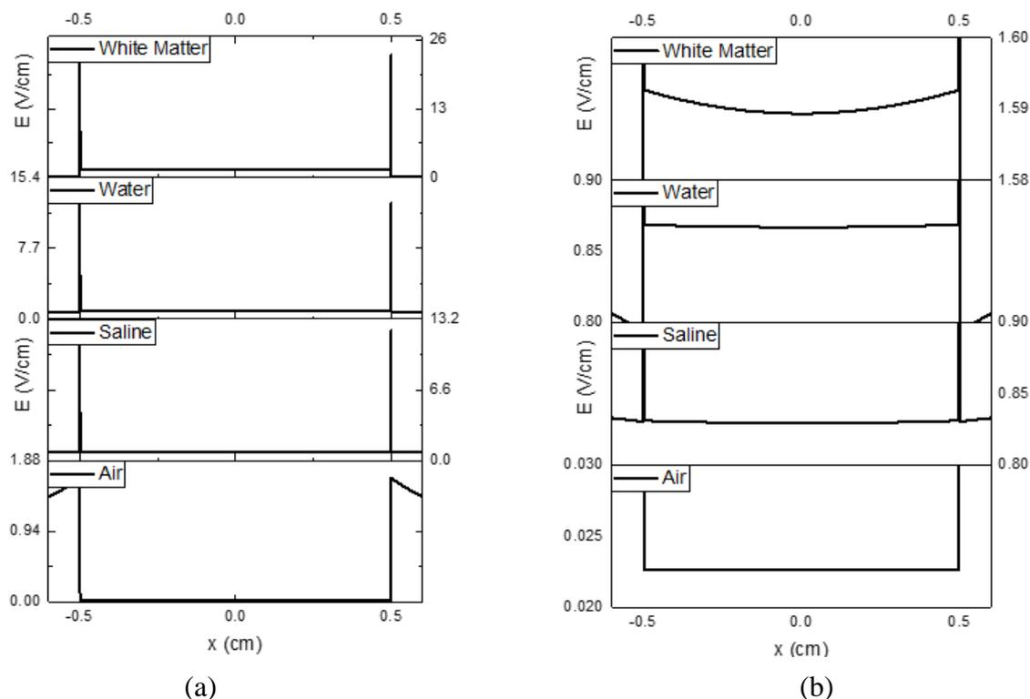
**FIGURE 3.** The EF intensity distribution on the lesion in various mediums with the radius of 1 cm and applied voltage difference between electrodes is 20 Vpp on a) lesion-medium boundary and b) inside the lesion.
