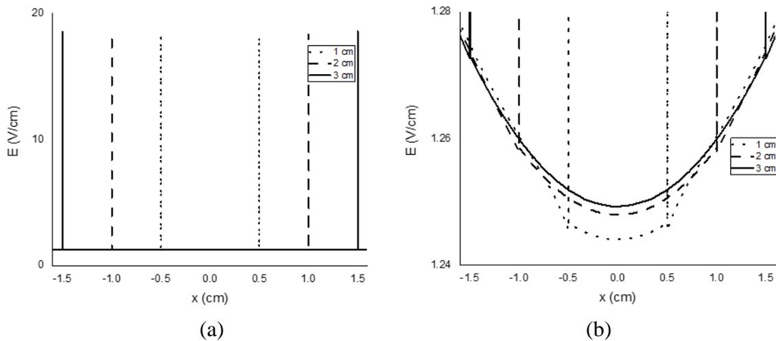
**FIGURE 5:** The distribution of the electric field intensity on lesion placed in a saline medium in various radius and applied voltage difference on both electrodes of 30 Vpp on: a) lesion edges and b) lesion interiors.
