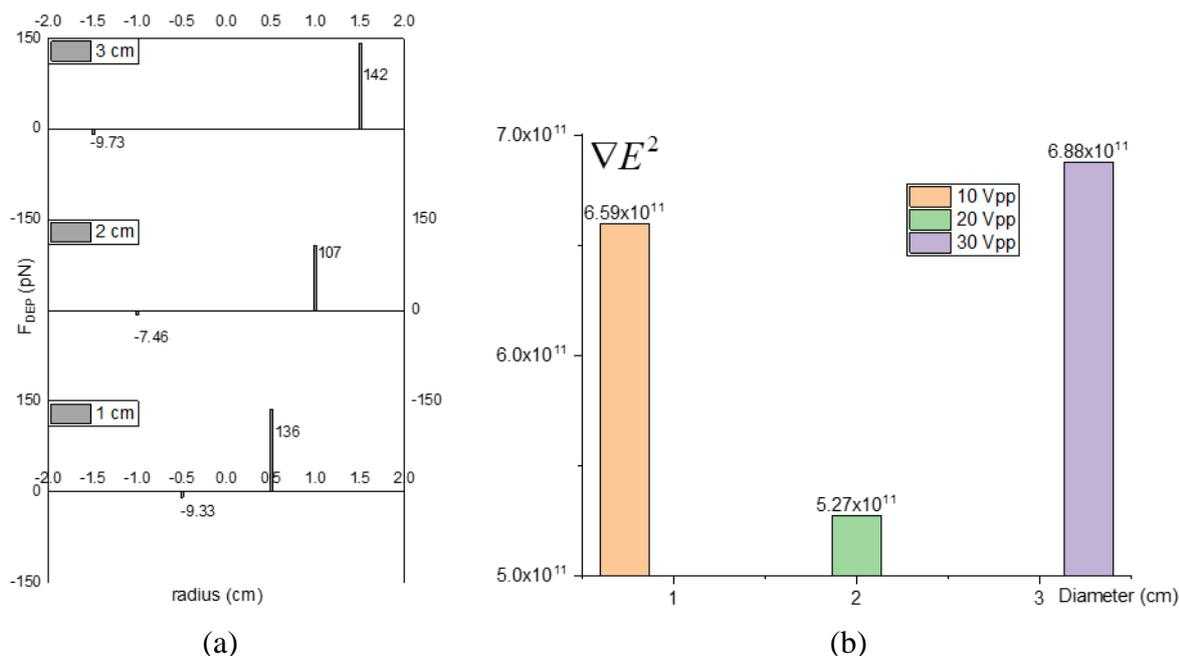
**FIGURE 8.** Dielectrophoretic forces at the lesion on the saline medium with an applied voltage difference between the electrodes 20 Vpp with various lesion diameter a) and their gradient of square electric field b).
