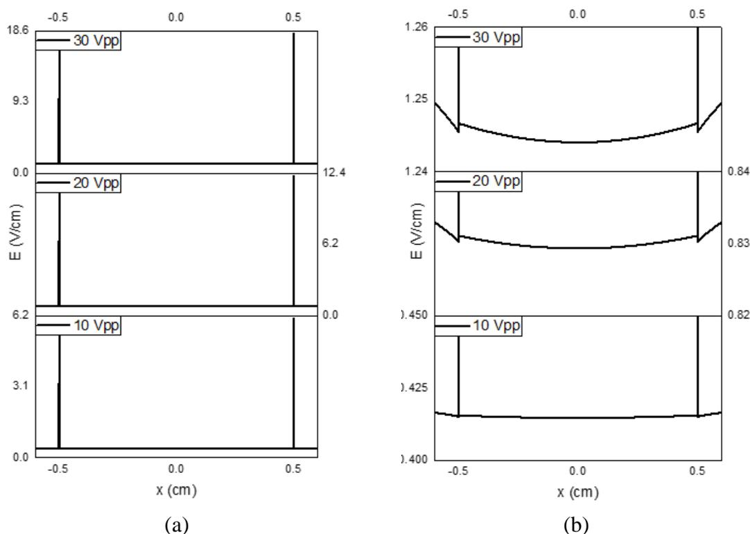
**FIGURE 4.** The distribution of the EF intensity with lesion radius of 1 cm surrounded by saline medium with various applied voltages difference (Vpp): a) lesion edges and b) lesion interiors
