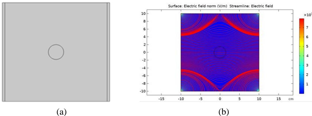
**FIGURE 2.** (a) Schematic diagram of the circular shape model of the lesion with 3 cm in radius inside the saline medium placed between applied voltages of + 15 V and -15 V (total voltage difference 30 Vpp) with medium dimension 20 cm x 20 cm; (b) Distribution of electric field intensity.
