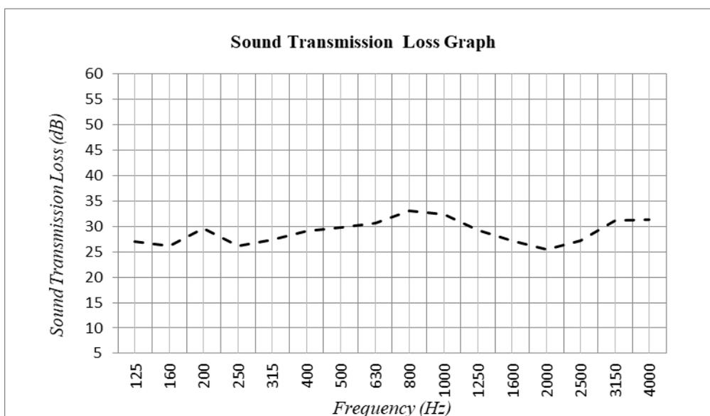
FIGURE 6. The STC on tempered glass at 10 mm thickness with lamination.
