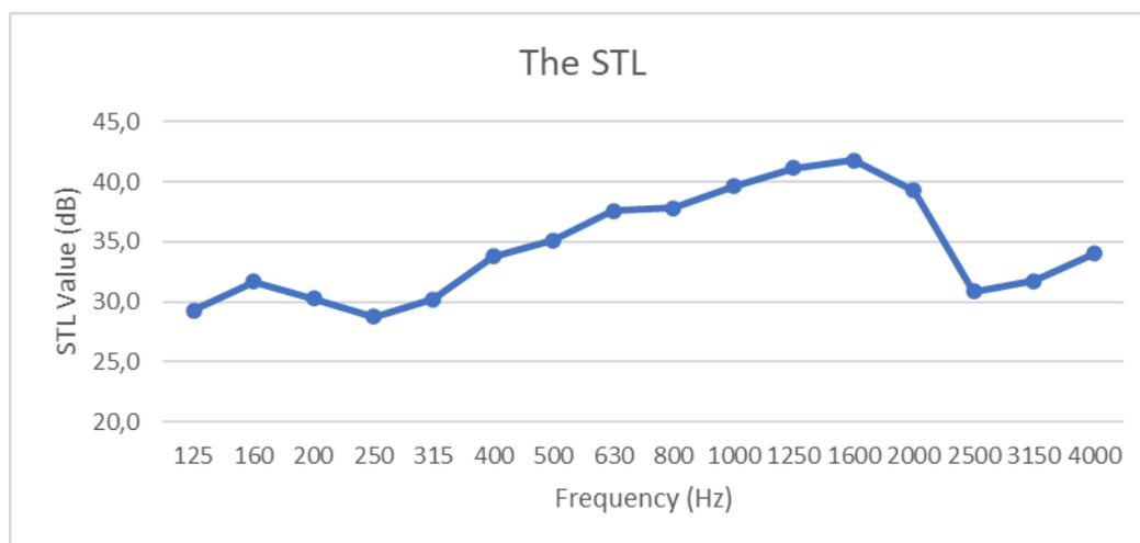
**FIGURE 4.** The SLT chart of 12mm tempered glass sample with lamination.
