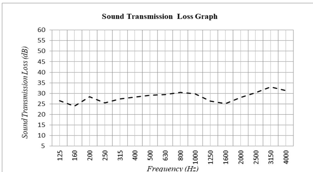
FIGURE 5. The STC on tempered glass at 10mm thickness.
