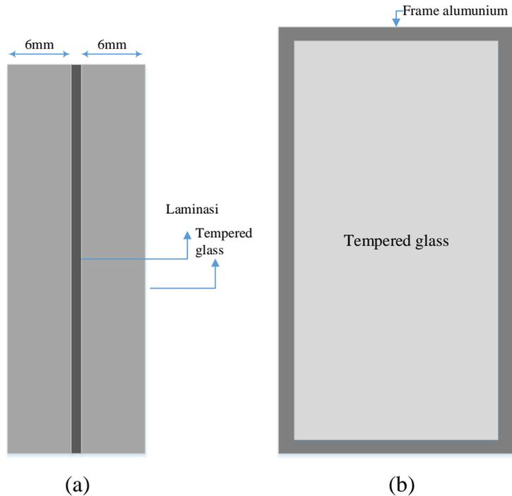
**FIGURE 3.** (a) Tempered Glass Laminated Side View (b) Tampered Glass Installation
