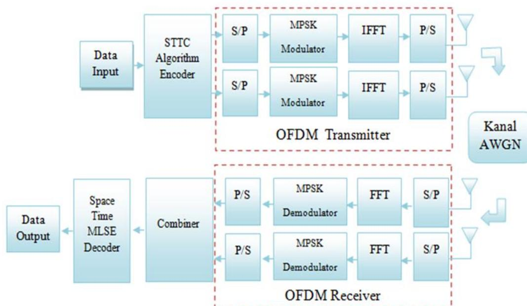
**FIGURE 5.** Block Diagram of STTC
