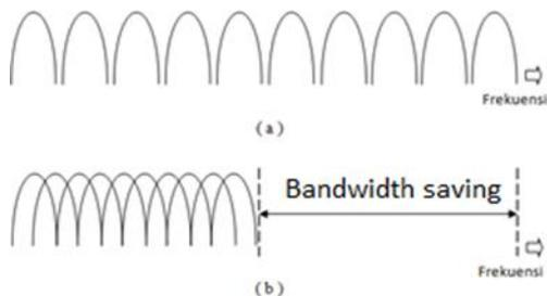
FIGURE 2. Conventional FDM Modulation Technique (a), OFDM Modulation Technique (b)
