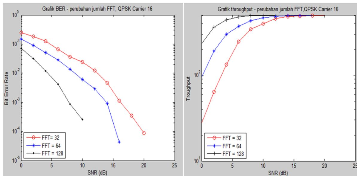
**FIGURE 9.** Graph of BER vs. SNR and throughput on the effect of changes in FFT on system performance with QPSK and carrier modulation16
