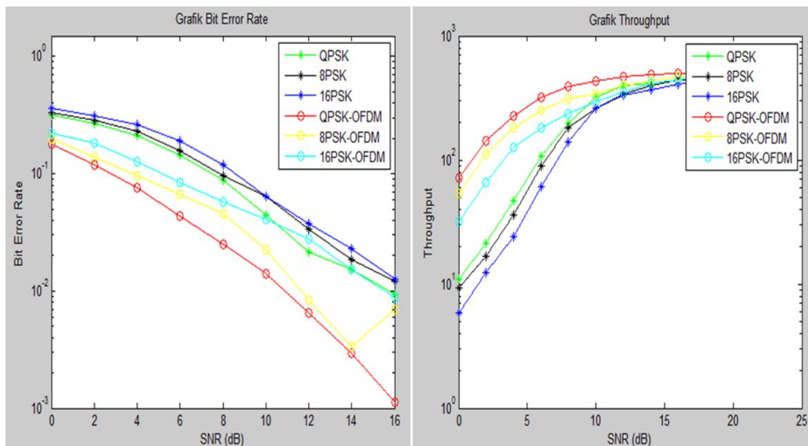
**FIGURE 7.** BER vs SNR and Throughput graph on the effect of OFDM usage on system performance with QPSK, 8PSK and 16PSK
