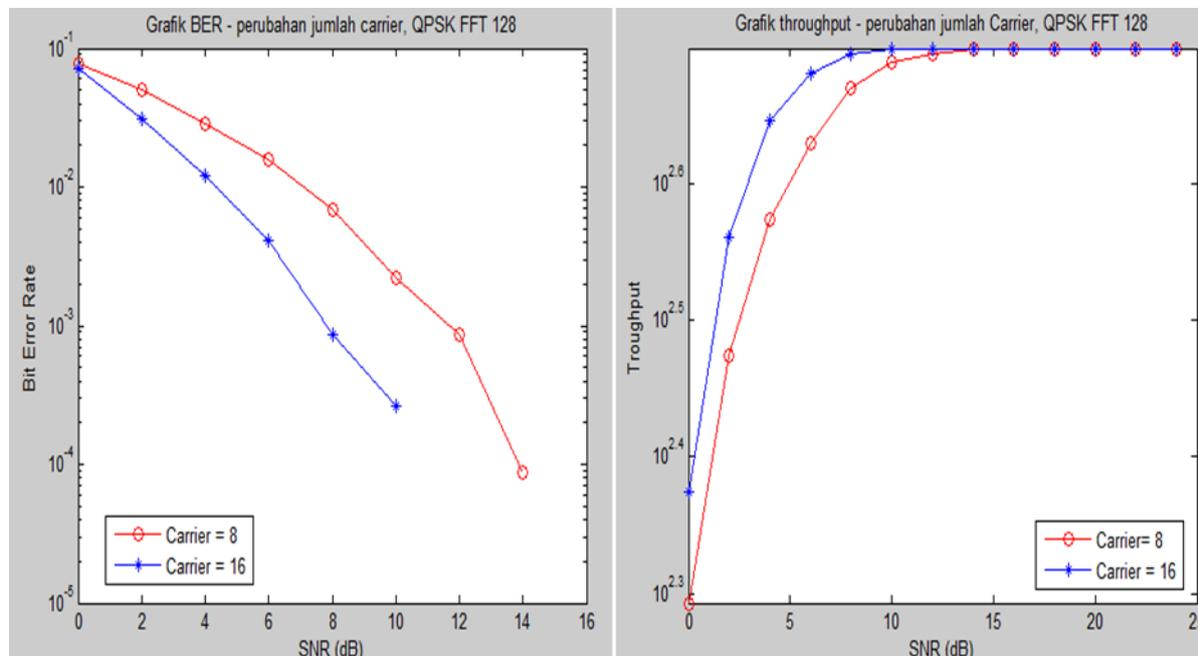
**FIGURE 8.** Graph of BER vs SNR and Throughput on the effect of carrier changes on system performance with QPSK and FFT128 modulation
