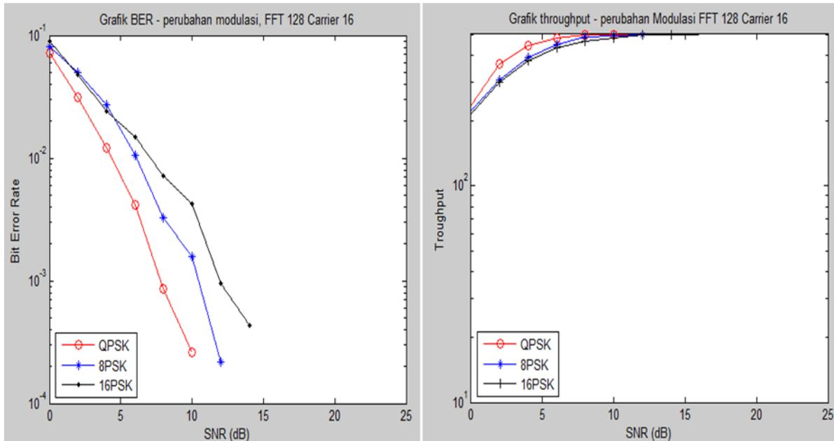
**FIGURE 10.** Graph of BER vs. SNR and throughput on the effect of changes in modulation on system performance with FFT128 and carrier 16
