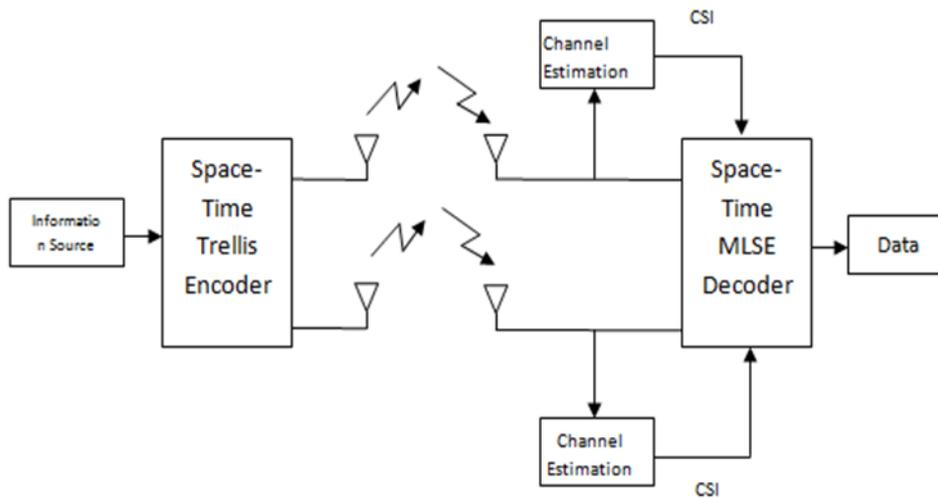
FIGURE 3. Block Diagram STTC[14]
