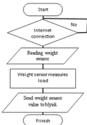
FIGURE 5. Weight sensor monitoring test flowchart
