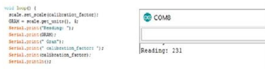
FIGURE 4. (a) snippet of the weight sensor reading program. (b) the results of the weight sensor readings under load.
