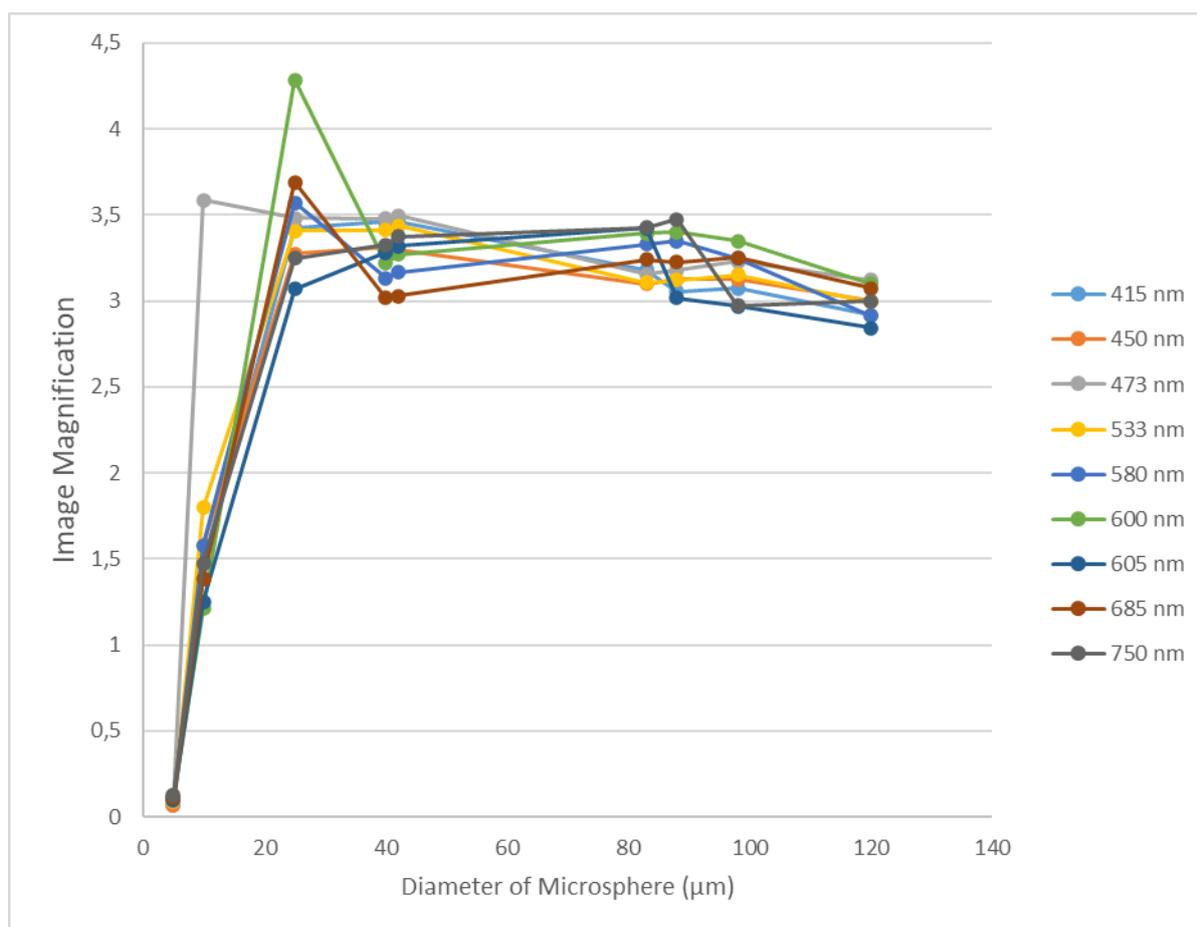
**FIGURE 4.** Image magnification as a function of microsphere's diameter for each light-source in visible light spectrum using soda-lime glass microsphere in free-space
