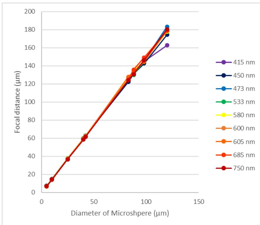
**FIGURE 3.** The position of maximum intensity of photonic jet (focal distance) generated by a barium titanate microsphere when illuminated by visible light as a function of the diameter of microsphere.
