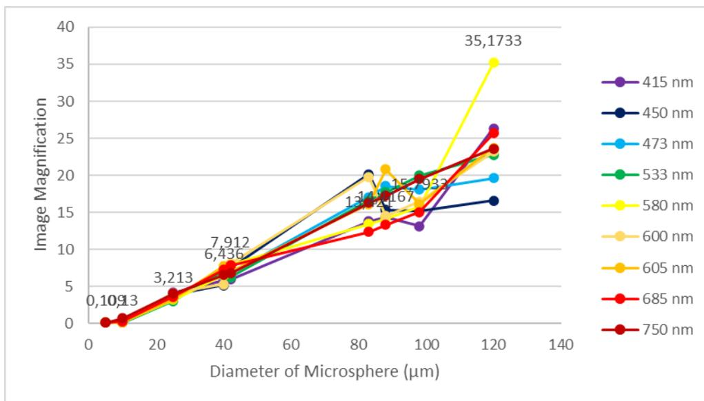
**FIGURE 2.** Image magnification as a function of microsphere’s diameter for each light-source in visible light spectrum using barium titanate microsphere in free-space. The largest magnification is yielded when the light-source has a wavelength of 580 nm (yellow).
