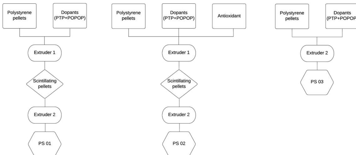
**FIGURE 1.** Schematic diagram of PS 01, PS 02 and PS 03 fabrication processes.
