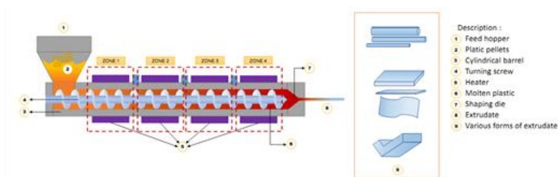
**FIGURE 2.** Schematic diagram of extruder machine number 1.
