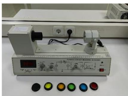
**FIGURE 1.** Photoelectric Effect Experiment Set
