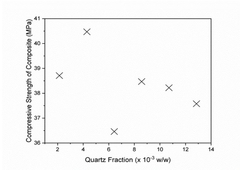
**FIGURE 5.** Compressive strength of mango leaf waste/PU/quartz composite as quartz content where the maximum strength of 40.47 MPa is attained at PU content of 0.06 (w/w).
