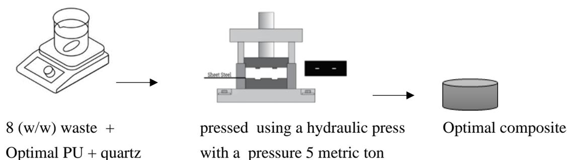
**FIGURE 2.** Diagram of the scheme of making mango leaf composites, PU and quartz.
