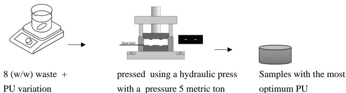
**FIGURE 1.** Diagram of the scheme of making mango leaf composites and PU variations.
