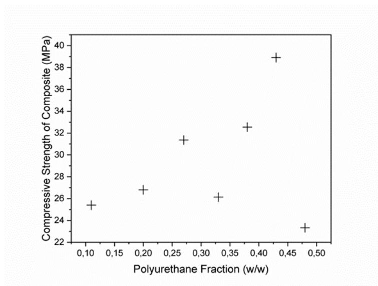
**FIGURE 4.** Compressive strength of mango leaf waste/PU composite as PU content where the maximum strength of 38.91 MPa is attained at PU content of 0.43 (w/w).
