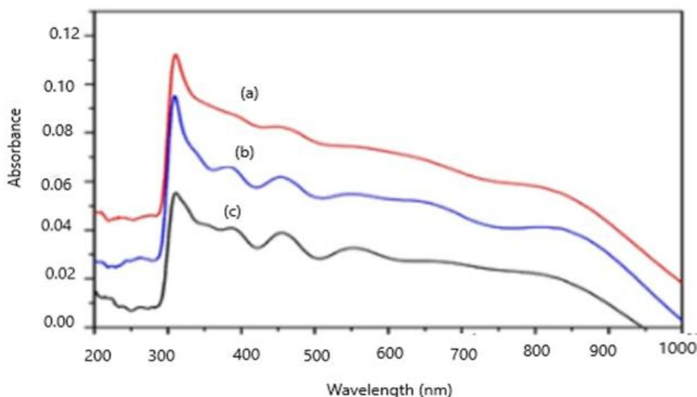
**FIGURE 4.** Spectrum of the  $0.3\text{BaTiO}_3 - 0.7\text{BaZr}_{0.5}\text{Ti}_{0.5}\text{O}_3$  thin film with (a) at  $700^\circ\text{C}$ , (b) at  $750^\circ\text{C}$  and (c) at  $800^\circ\text{C}$
