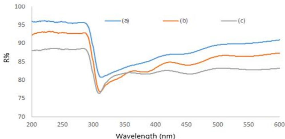
**FIGURE 3.** UV-Vis reflectance curve of  $0.3\text{BaTiO}_3 - 0.7\text{BaZr}_{0.5}\text{Ti}_{0.5}\text{O}_3$  thin film annealed at (a)  $700^\circ\text{C}$ , (b)  $750^\circ\text{C}$  and (c)  $800^\circ\text{C}$ .
