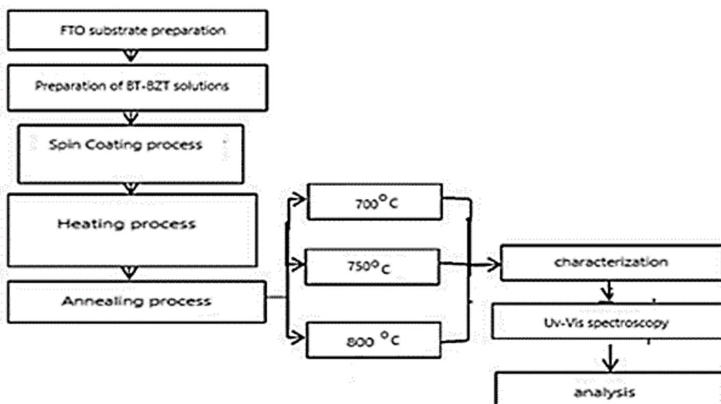
FIGURE 2 : Flow chart making of thin film BT-BZT.
