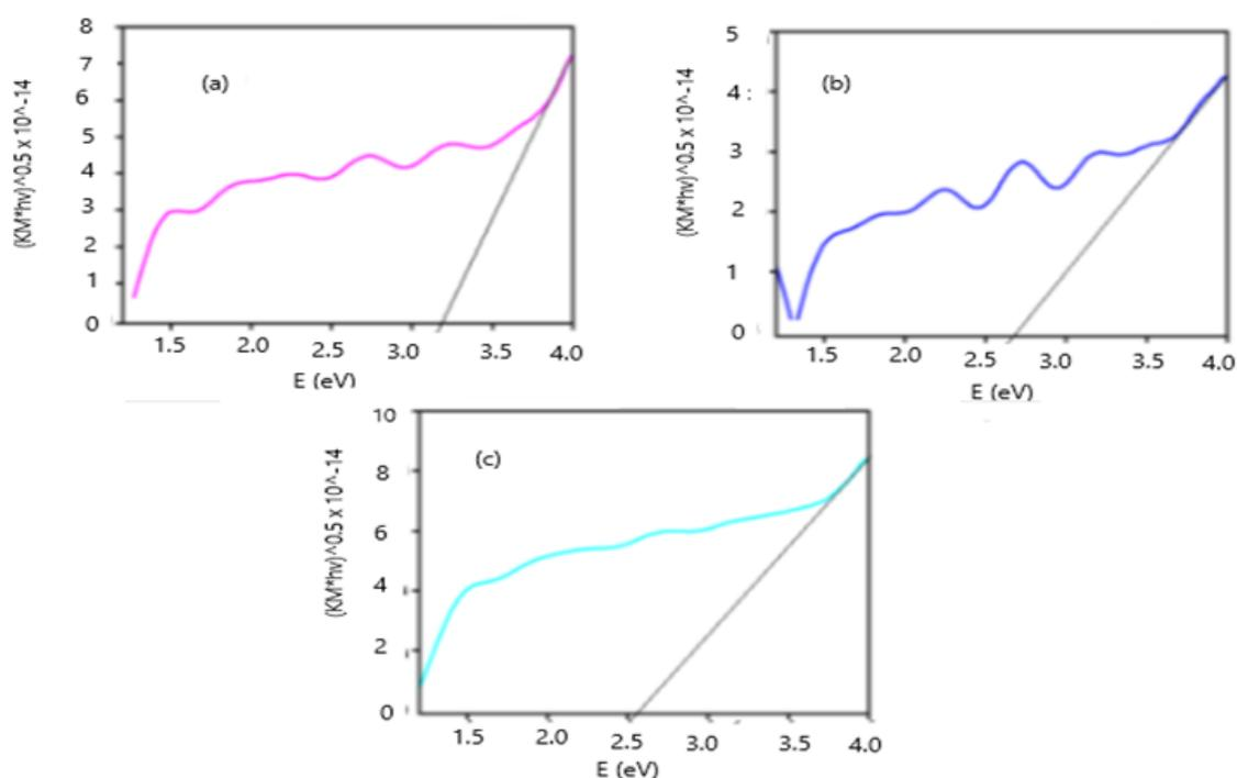
**FIGURE 5.** Determination of  $E_g$  Value from the relationship  $(F(R)hv)^{\frac{1}{2}}$  and  $hv$  Energy (eV), (a) at  $700^\circ\text{C}$ , (b) at  $750^\circ\text{C}$  and (c) at  $800^\circ\text{C}$
