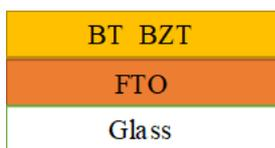
FIGURE 1. BT-BZT Thin Film Structure
