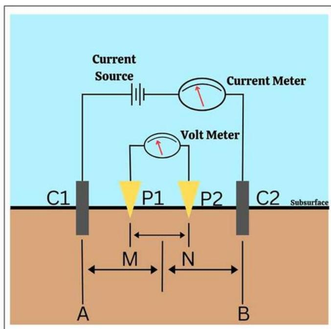
**FIGURE. 2.** Schlumberger electrode configuration array
