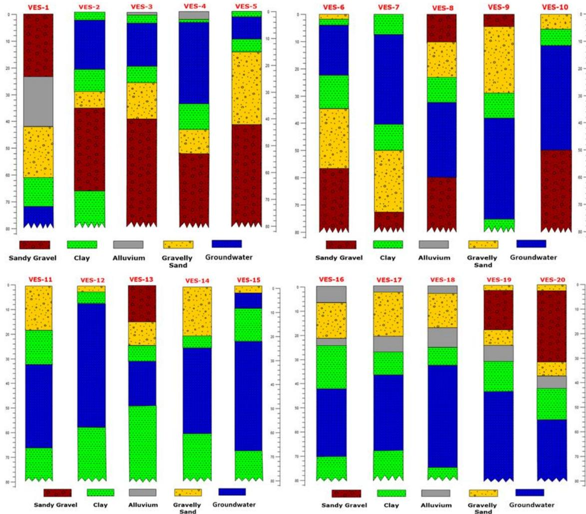
FIGURE 4. Model of the geological and geoelectrical sections at each of the twenty VES points.
