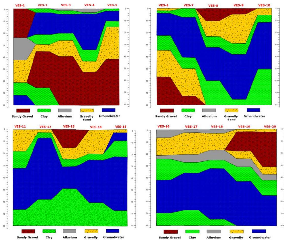
**FIGURE 5.** The twenty locations of the VES and their geoelectric correlation.
