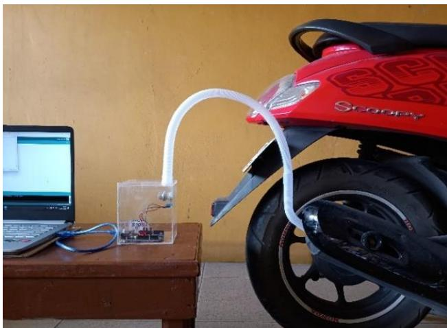
FIGURE 3. Vehicle's exhaust gas sensing measurement setup.
