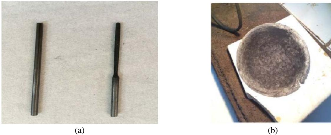
**Figure 2.** (a) graphite pencil before (left) and after (right) the electrolysis process, (b) the powder obtained after filtering and purification process.
